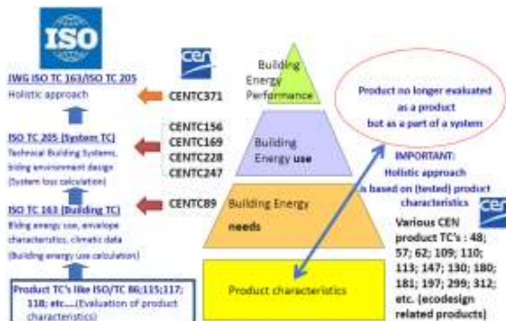
Figure 3-5 Hierarchical range of scope of technical standards from product/ component level to overall system level
