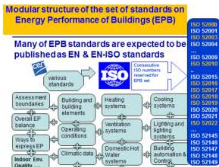
Figure 3-2 Modular structure and interaction of European standards on energy performance of buildings
